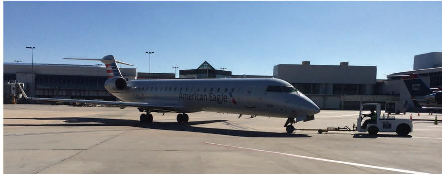
As per the Caution box on the top of 4-34 of the EGOM, Pushback must start in a SLOW, SMOOTH, and CONTROLLED motion. NO jerking motions or sudden stops as this will damage the aircraft. Not only could this have caused damage to the aircraft, but flight attendants are typically standing at the time of pushback and this could cause severe injury to the flight attendants or the passengers onboard.
