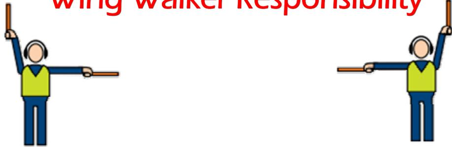
The primary responsibility of a wing walker is to ensure there is enough clearance between the aircraft and any obstacle.
